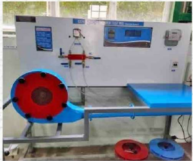
Centrifugal Blower with data logging facility
