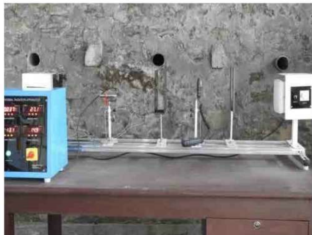
Radiation Apparatus with Radiation Shield Arrangement
