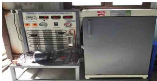
VCR Test Rig (domestic refrigerator) -Manual Mode
