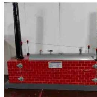
Cut-section Model of Lancashire Boiler
