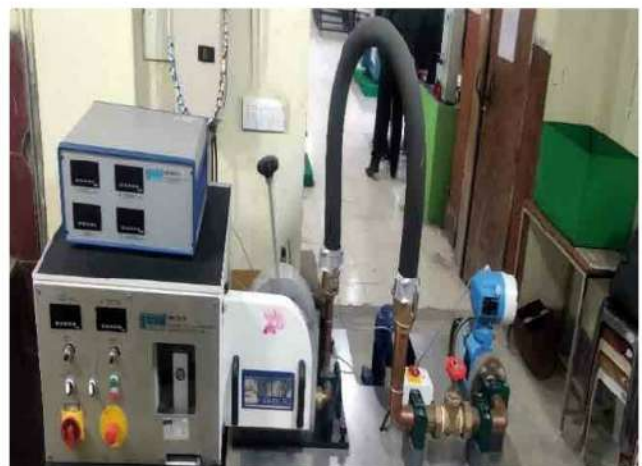
Turbines (Pelton and Francis) Test-Rig
