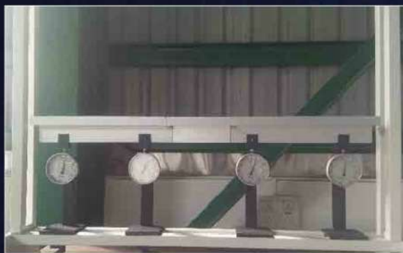
Line of Influence on the Gerber Beam
