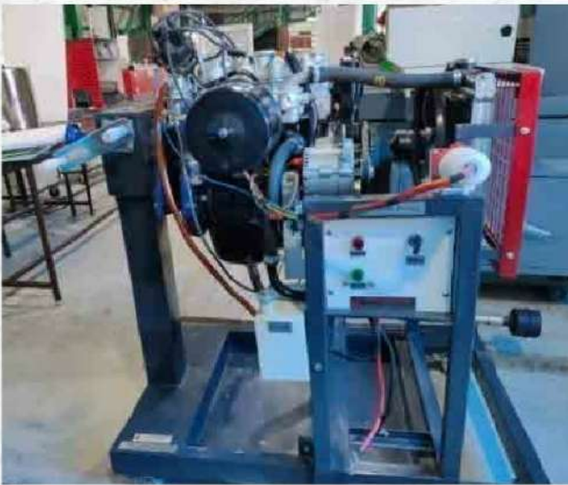
Assembling and dismantling set-up of 4-S 4-C Petrol Engine (working)
