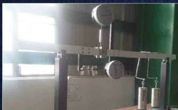
Beam on two support Shear Force &amp; Bending Moment
