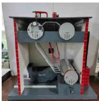
Cut-section Model of Stirling Boiler
