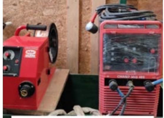
**Metal Inert Gas (MIG) Welding Setup**
