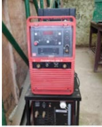
**Tungsten Inert Gas (TIG) Welding Setup**
