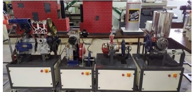
Cut section Models of Engines and Boilers
