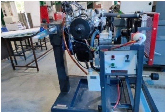
Assembling and dismantling set-up of 4-S 4-C Petrol Engine (working)
