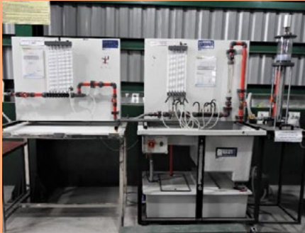
Flow Measuring Device
