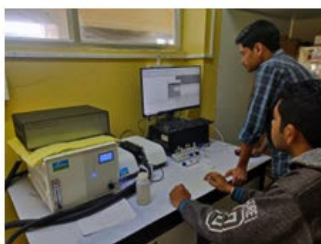
Diode array Spectrophotometer with Peltier
