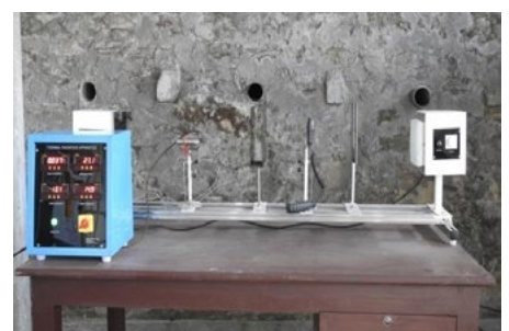
Radiation Apparatus with Radiation Shield Arrangement
