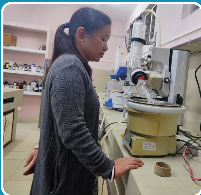
Ms. Srijana Subba, PhD scholar using rotary evaporator for synthetic organic chemistry research.
