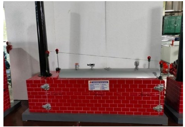
Cut-section Model of Lancashire Boiler
