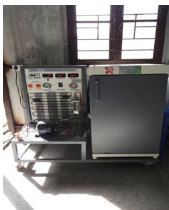
VCR Test Rig (domestic refrigerator) -Manual Mode
