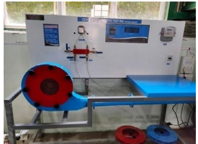
Centrifugal Blower with data logging facility
